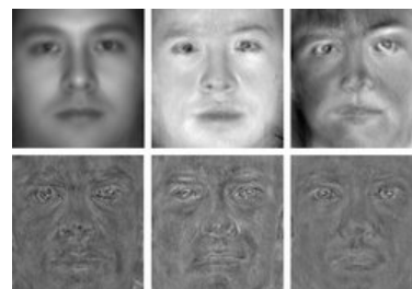
Figure 10: Some eigenfaces. Top left is the mean face image, and the other two images on the top row are the first two principal components (“eigenfaces”). The bottom row shows the three smallest principal components: these supposedly contain the least amount of information. [Scholarpedia article on eigenfaces 2009]
